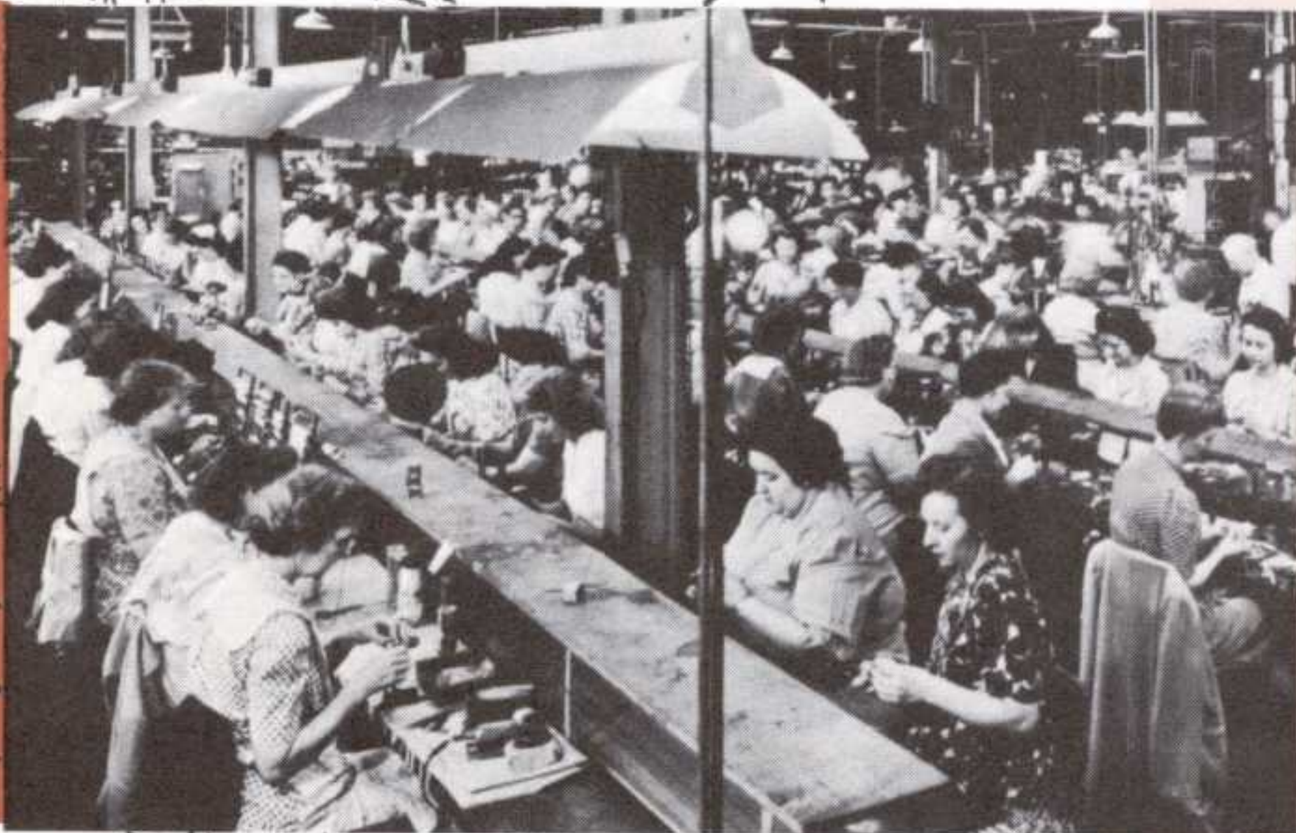
One of several CHICAGO assembly departments. Here, insulated leads are attached to the coil, and laminations inserted around the coil to form the core
