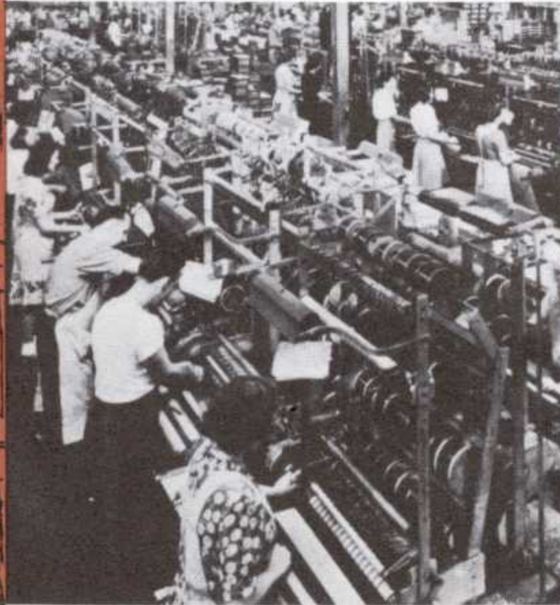
A section in one of CHICAGO's coil winding departments. Each machine winds up to 30 coils to a spindle simultaneously
